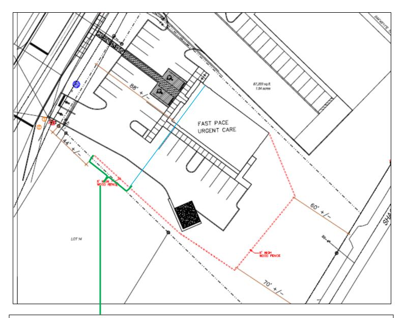
This section of fence is non-compliant. Per Article 10.3.L, from five feet behind the front building line forward to the front lot line and in the corner side yard, privacy fences and walls are limited to 42 inches. The beginning of the fence starts at 44' from property line. This section is 51' (to where the 5' behind the front façade line starts) and non-compliant.
