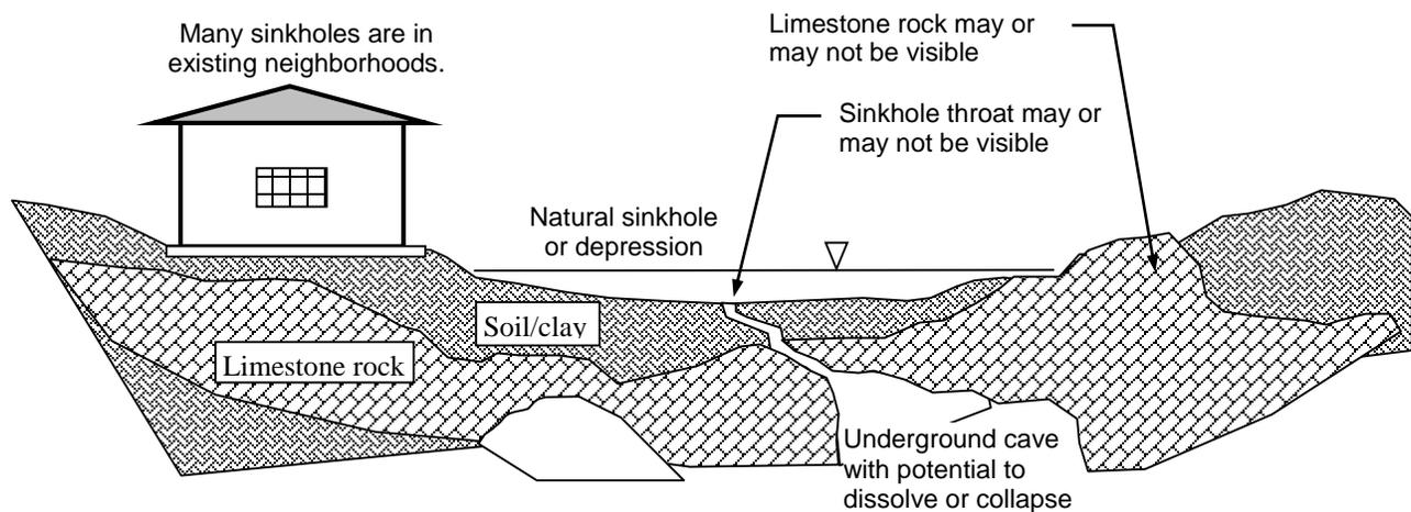
Increasing stormwater runoff to a natural depression may increase sinkhole formation by further dissolving limestone. Even if the amount of stormwater runoff has not been increased, stormwater quality treatment is necessary to prevent pollutants from entering groundwater and to reduce potential pH changes and chemicals within stormwater runoff.
